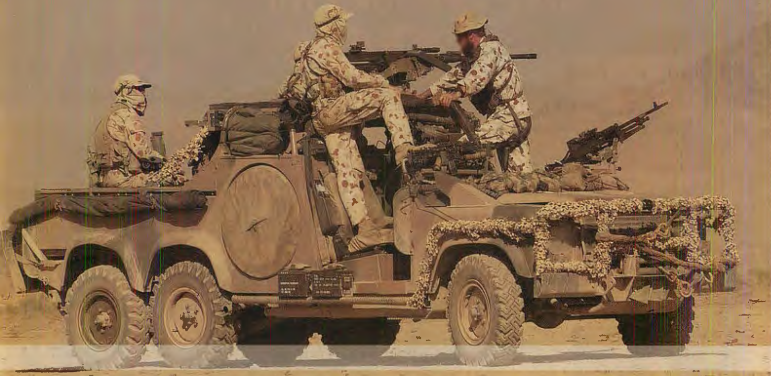
Side view shot of the SAS 6x6 long range patrol vehicle in Afghanistan showing both the .50 calibre and 7.62 mm general purpose machine gun.
